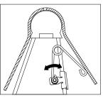
Figure E2: Cutaway view of driver side pivot arm and saddle.
