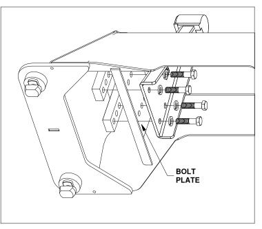
Figure A2: Passenger pivot arm mounting location.
