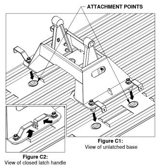
Adjust the tension in the latch handle, for parts list and visual guide refer to Figures C3 and C4.
