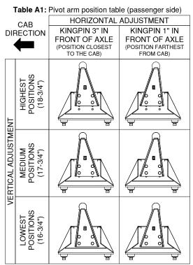
▲ WARNING: B&W recommends that you check the clearance between the truck cab and the trailer. Compare the measurement taken from the center of the Coupler to the cab, to the measurement taken from the center of the king pin to the farthest forward corner point of the trailer. These measurements will allow you to see how much clearance you will have between the cab and the trailer while towing and turning.
