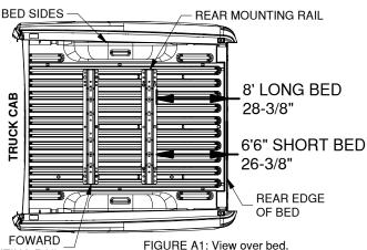
**IMPORTANT:** The mounting rail is designed to install only at the described location. Failure to place the mounting rail precisely may result in added difficulty during installation and/or property damage.
