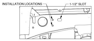
Figure F1: View looking into driver side wheel well.
