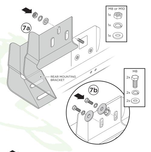
**8a.** If installing Rear Mounting Bracket WITH Rear Support Brace, position Rear Support Brace over the Rear Mounting Bracket and attach the top mounting point to the vehicle using M8 or M10 hardware depending on bolt plate used. You will use one (1) Flat Washer, one (1) Lock Washer and one (1) Hex Head Nut.
