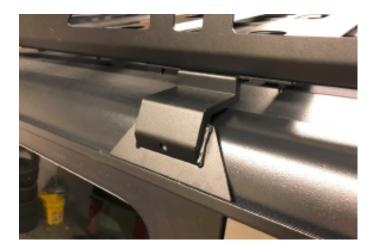
6. Install outer clamp to the roof bracket. Attach with 4 longer button head bolt and washer.
