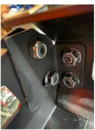
2. Slide the 3 center braces into place and attach with hardware. Use the longer button head bolts with 2 washers and Nyloc nut. Snug all the hardware but don't fully tighten at this time. With it only snug, it allows you to adjust the roof bracket when placing it on the Jeep later.
