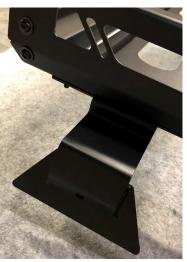
3. Attach the front panel to the rack using the Corner Braces. The Corner Braces will install from the inside. Use the short button head with 2 washers and Nyloc nut. With the rack assembled, fully tighten all the hardware except the hardware holding the roof brackets. These feet need to stay flexible to adjust to fit to the roof. **NOTE**: At this time attach LED cubes to the front panel if you choose.
