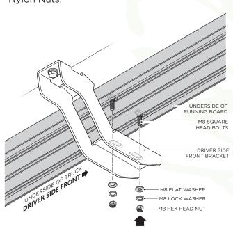
**6.** Fasten the Running Board to the Driver Side Center Bracket cradle by using (2) M8 Flat Washers, (2) M8 Lock Washers and (2) M8 Nylon Nuts.
