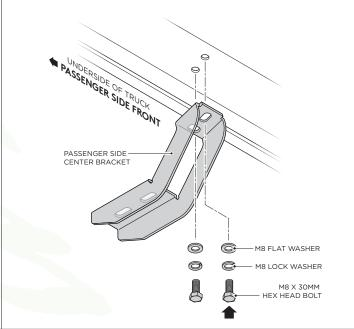
**4.** Fasten the top portion of the Passenger Side Rear Bracket by using (2) M8 x 30MM Hex Head Bolts, (2) M8 Flat Washers and (2) M8 Lock Washers.
