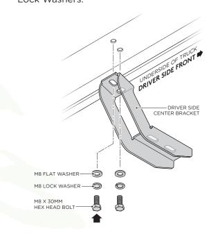
**4.** Fasten the top portion of the Driver Side Rear Bracket by using (2) M8 x 30MM Hex Head Bolts, (2) M8 Flat Washers and (2) M8 Lock Washers.
