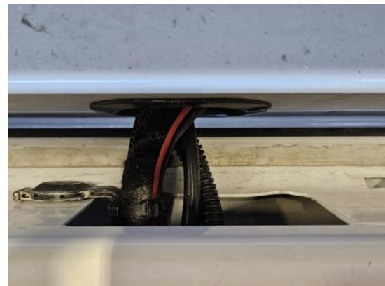
20. Connect the plug and plays 4-pin connector and the light bars 4-point connector as well as the weatherpack connectors.
