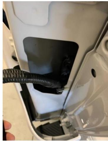
4. Disconnect the factory harness from the taillight. Now plug the female end of the in the Putco quick disconnect harness into the tail lamp and the male harness into the factory harness. The taillight can be reattached to the truck.
