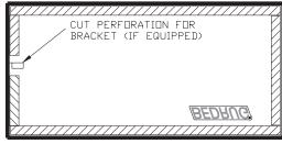
**NOTE:** Cut opening at perforation if tailgate has metal arm.
