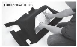
6. Cut the hook fasteners with tape backing to match the length of the loop sewn on the underside of each BedRug/BedTred piece. Pre-install provided heat shields on underside of the two front pieces in areas using the locator marks. (Fig. 1) Note: Passenger side heat shield is the larger of the two pieces.
