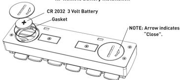
Install the Cr2032 batteries as shown. Be sure to turn the battery door to the right (clockwise) to open, the arrows indicate the direction to close (counter clockwise).
