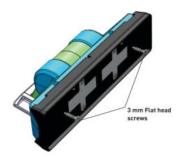
Installation of Trigger Mounting Plate
