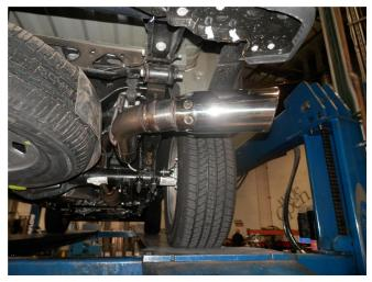
**Step 3.** Loosely attach the Tail Pipe Assembly using a similar fashion. Keep all fasteners loose for final adjustment.
