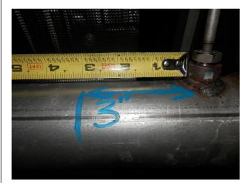
**Step 1.** Begin removal by removing the secondary O2 sensor at the over axle pipe of the OEM system. Next, cut the OEM inlet pipe 3.00" rearward of the O2 sensor behind the
