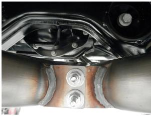
**Step 3.** Next attach the Mid-Pipe Assemblies to the Resonator Assembly using the supplied 2.50" clamps. At this time also use the supplied 5/16" fasteners to connect the Mid Pipe Assemblies.
