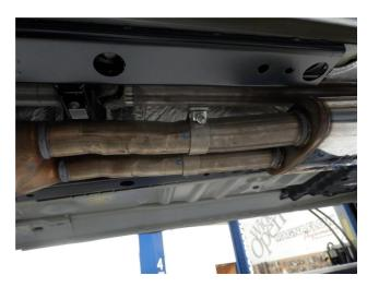
**Step 2.** To install the new Magnaflow exhaust system begin by attaching the Resonator Assembly to the cut and de-burred outlet of the OEM system using the supplied 2.25" clamps. Leave all clamps loose until final adjustment of the system.
