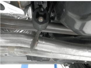
**Step 1.** To remove the OEM exhaust begin by cutting the tubing at the weld junctions in front of the OEM resonator. Once cut, working front to rear, disengage the hangers from the rubber insulators and remove the system. Do not damage or discard the rubber insulators as they will be re-used to install the new Magnaflow system.
