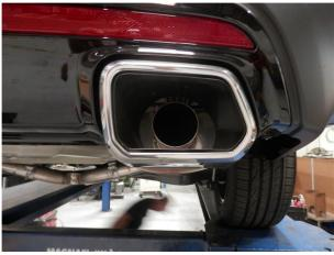
**Step 4.** Complete the installation by attaching the Muffler Assemblies to the Mid-Pipes using a 2.50" clamps and fitting the tailpipes into the openings in the rear valance and the hangers into the rubber insulators.
