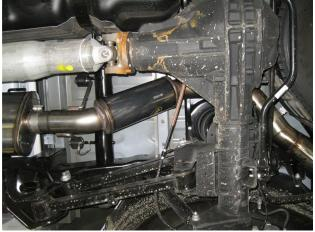
**Step 2.** Begin by attaching the Muffler Assembly to the factory outlet and the Resonator Assembly to the Muffler Assembly outlet using the supplied 3.50" clamps. Fit the hangers into the rubber insualtors. Leave all clamps loose until final adjustment.
