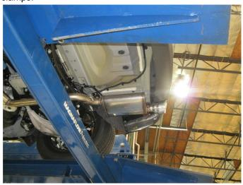
**Step 4.** Install the Muffler Tail Pipe Assembly in a similar fashion using the remaining 2.50" clamp. Locate all welded hangers to the rubber insulators.
