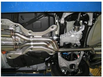
**Step 3.** Loosely install the Y-Pipe Assembly to the two Resonator Assemblies using two of the suppled 2.50" clamps.
