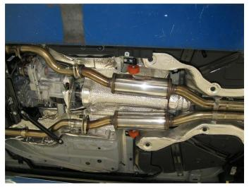
**Step 2.** Begin installing your new system by first loosely attaching both Resonator Assemblies to the vehicle outlet flanges using the four supplied M10 bolts.
