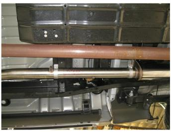
**Step 3.** Install the Mid Pipe Extension Assembly using the supplied 3.50" clamp. Use the supplied 19.25" Extension Pipe between the Inlet Y-Pipe Assembly and the Mid Pipe Extension Assembly if your truck has a long bed configuration.
