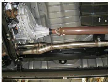
**Step 2.** Install the new system by attaching the Inlet Y-Pipe Assembly to the OEM catalytic converter outlet pipes using the existing clamp and hardware. Locate the welded hanger to the rubber insulator. Leave all clamps and fasteners loose for final adjustment of the complete system once installed.
