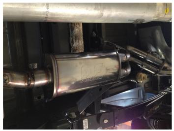
**Step 3.** Install the Muffler Assembly to the Inlet Pipe Assembly using the supplied 3.00" clamp.
