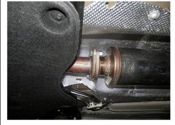
**Step 3.** Begin installation of your new MAGNAFLOW system by attaching the Inlet Muffler Assembly to the catalytic converter outlet using the OEM nuts and supplied bolts. Keep all fasteners and clamps loose until final adjustment.
