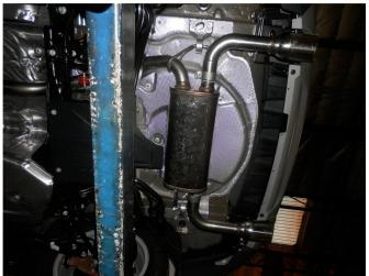
**Step 5.** Loosely attach the Muffler Assembly and the two Tail Pipe Assemblies using the supplied 2.25" clamps in a similar fashion,
