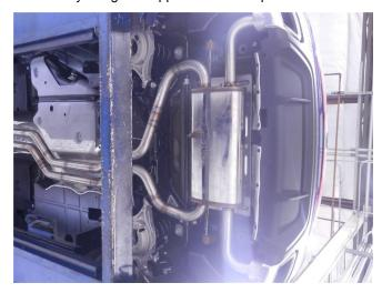
**Step 4.** Finish the installation by fitting the Muffler Assembly onto the Mid pipes using the supplied 2.25" clamps and inserting the hangers into the rubber insulators. The tailpipes will fit into the stock exhaust openings in the rear valance
