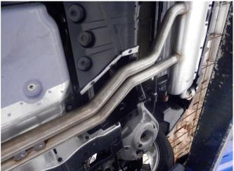
**Step 1.** Begin removing the OEM exhaust system by loosening the clamps located in front of the resonator. Next working front to rear extract the hangers from the rubber insulators and remove the OEM system. Retain insulators as they will be used to install the new system.
