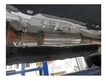
**Step 2.** To install the new Magnaflow exhaust system begin by attaching the Resonator Assembly to the cut and de-burred outlet of the OEM system using the supplied 2.36" clamp. Leave all clamps loose until final adjustment of the system.
