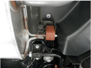
**Step 1.** To remove the OEM exhaust begin by cutting the tubing approximately 2.00" behind the weld on the catalytic converter. Once cut, working front to rear, disengage the hangers from the rubber insulators and remove the system. Do not damage or discard the rubber insulators as they will be re-used to install the new Magnaflow system.
