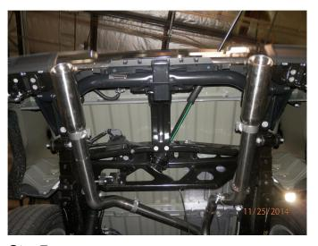
Step7. Install the two Clamp-On Tips using the supplied 2.50" clamps.
