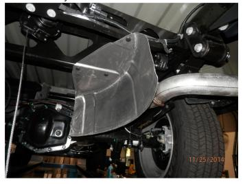
**Step 2.** You will also need to remove the spare wheel and heat shield.
