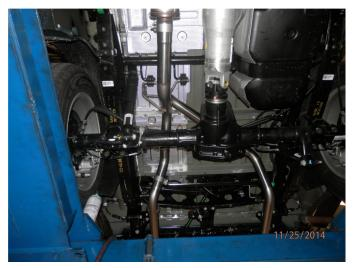
**Step 5.** Continue the installation by loosely attaching the Over Axle Assemblies to the Muffler using a supplied 2.50" clamp and inserting the hanger into the rubber insulator.
