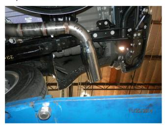
**Step 4.** Complete the installation by attaching the Tail Pipe Assembly to the Muffler using a supplied 3.00" clamp and inserting the hanger into the rubber insulator.
