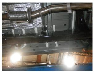
**Step 2.** Begin installing of the new system by attaching the Inlet Pipe Assembly to the flange re-using the OEM fasteners and inserting the hanger into the rubber insulator.
