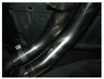
**Step 3.** Next Install the Tail Pipe Assembly to the Extension Pipes in a similar fashion using the supplied 3.50" clamps and by fitting the welded hangers into the rubber insulators.
