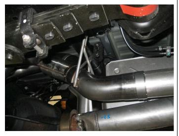
**Step 2.** Begin installation of the Magnaflow system by first clamping the Y-Pipe Assembly inlet to the newly cut outlet of the DPF using the supplied 4.00" clamp. Then attached the two Extension Pipes to the Y-Pipe Assy using the suplied 3.50" clamps and fitting the hangers in the rubber insulators (leave all clamps loose for final adjustment of the complete system). If your vehicle has an O2 sensor re-install at this time. If not, install the provided sensor boss plug.
