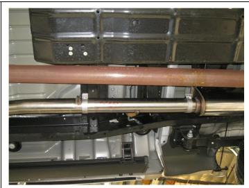
**Step 3.** Install the Muffler using the supplied 3.50" clamp. Use the supplied 16.00" Extension Pipe between the Muffler and the Tail Pipe Assembly if your truck uses the Crew Cab Long Bed or the Extended Cab Short Bed configuration. If your truck has a Crew Cab with the Short Bed the 16.00" Extension Pipe is not used.
