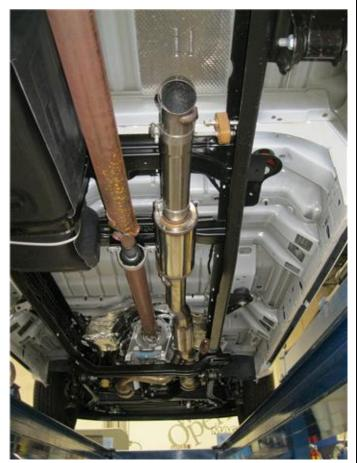
**Step 5.** Once a final position has been chosen for the new exhaust system, evenly tighten all clamps from front to rear using the torque specifications on page one of the instructions. Inspect all fasteners after 25-50 miles of operation and re-tighten if necessary.
