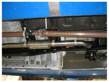
**Step 4.** Install the Muffler, Tail Pipe Assembly and Extension Pipe Assembly (if needed) using the supplied 3.50" clamps. Locate the welded hangers to the OEM rubber insulators.
