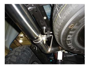
**Step 2.** Before installing your new system, to convert the vehicle to dual tips you must install the supplied threaded hanger into the driver side frame rail with the supplied fasteners as shown.
