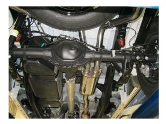
**Step 4.** Working front to rear install the remaining pieces of the MAGNAFLOW system, inserting hangers into rubber insulators and loosley intstalling suppled clamps. Adjustable tips are supplied to fit a variety of aftermarket bumpers and rollpans, once a position is decided for the tips it is recommended to have them welded into place.
