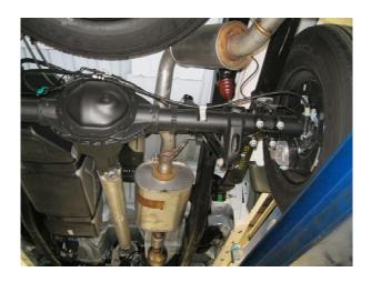
**Step 1.** To remove the OEM exhaust system, you will first need to cut the pipe behind the muffler before it goes over the axle. You can then disengage the welded hangers from the rubber insulators and remove the tailpipe. Unfasten the muffler inlet from the catalytic converter at the clamp junction. Do not damage or discard the OEM fasteners or rubber insulators, as they will be reused to mount the new system. Disengage the muffler hangers and remove it from the vehicle.
