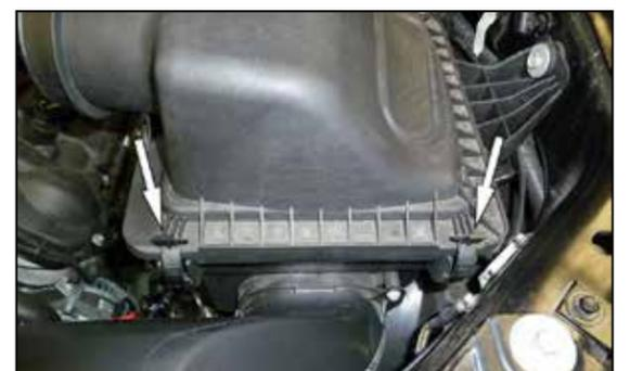
6. Release the two locking clips that secure the upper air filter housing and then remove the upper housing from the vehicle.
