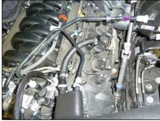
25. Connect the 90° fitting to the valve cover and the straight fitting to the fitting installed into the K&N® intake tube. Connect the EVAP vent line to the fitting installed into the K&N® intake tube.
