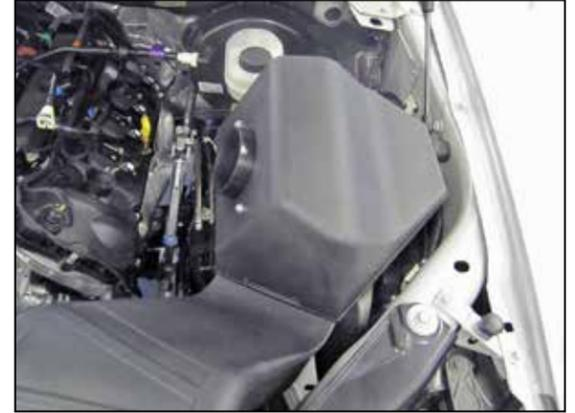
18. Install the upper air filter housing assembly onto the lower filter housing.
