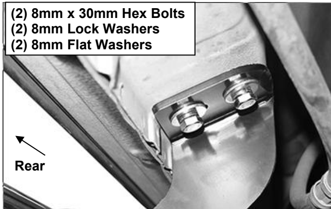
(Fig 7) Driver/Left Rear Bracket Pictured(Example Only)
