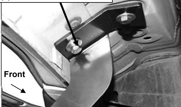
(Fig 3) Driver/Left Front Mounting Location Pictured
