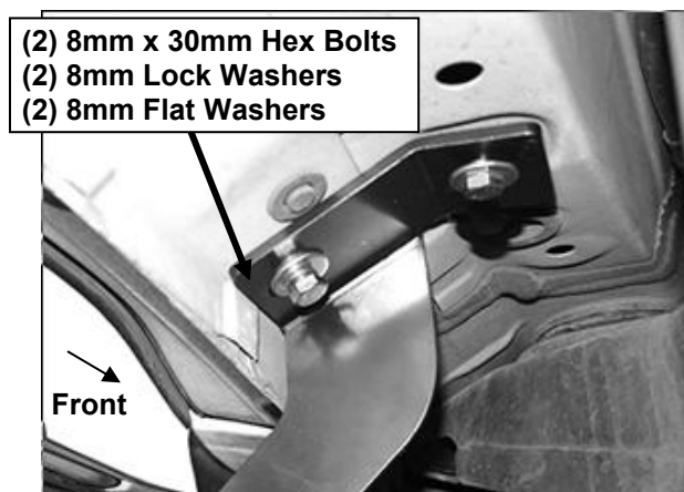
(Fig 3) Driver/Left Front Mounting Location Pictured
