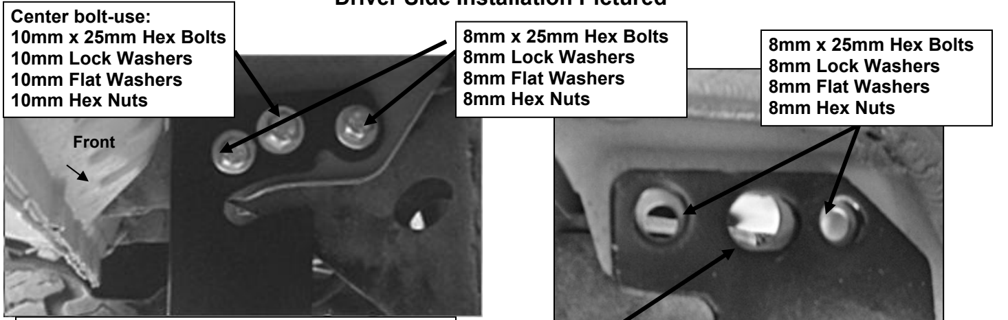
(FIG 1) Driver Side Front Mounting Location
