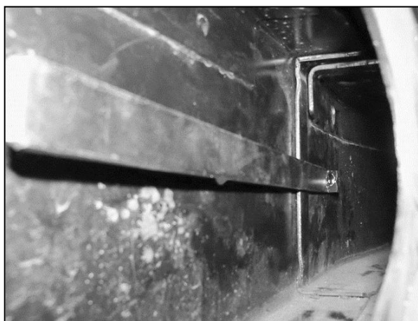
(Fig 3A) Inside view of Long Bolt Plate installed in driver side frame channel
