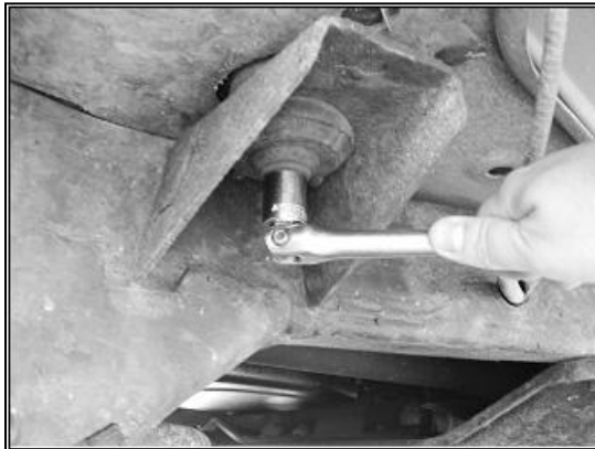
(Fig 1) Remove factory body mount bolt
