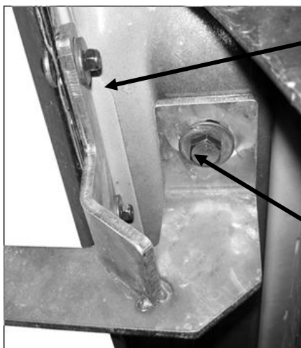
(Fig 3A) Passenger side Front Mounting Bracket installation pictured ("mid length" bracket)
