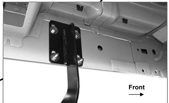
(Fig 5A) Front Bracket installation pictured
