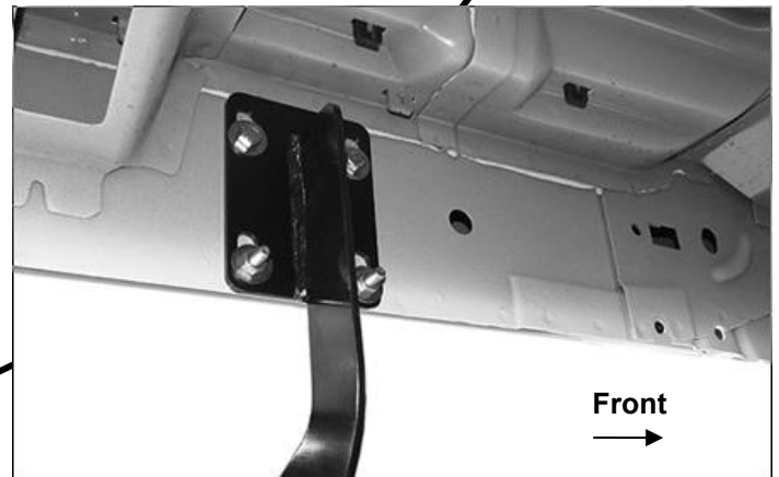
(Fig 5) Front Bracket installation pictured
