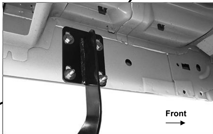
(Fig 5A) Front Bracket installation pictured
