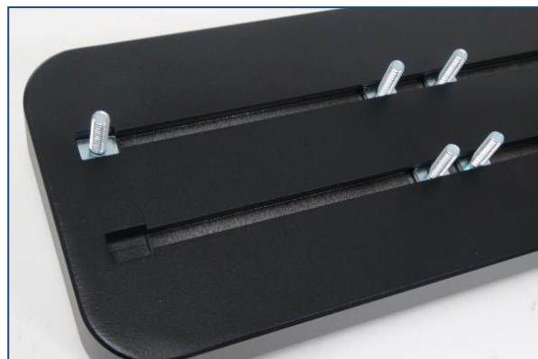
FIGURE 4 Slip M6 Square Head Bolts into channel
