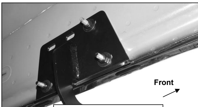
(Fig 3) Driver/left front side Mounting Bracket installed
