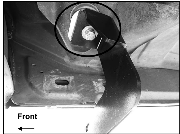
(Fig 3) Passenger/front Upper Bracket installation
