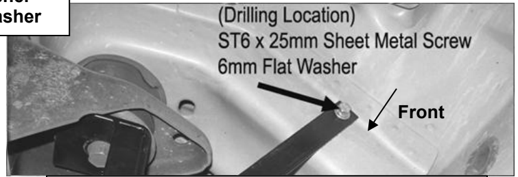
(Fig 3) Front Support Bracket(short) installation
