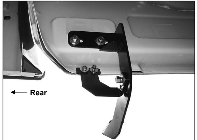
(Fig 16) Driver/Left rear Mounting Bracket assembly
