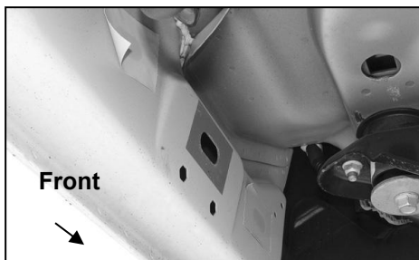
(Fig 1) 2009-mid 2015 Driver/Left front mounting location (No factory holes in pinch weld 2009-2011 models)
