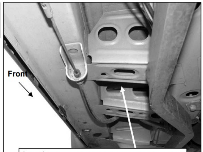
(Fig 5) Driver side center mounting location
