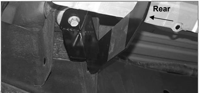
(Fig 9) Passenger side Rear Bracket Installation
