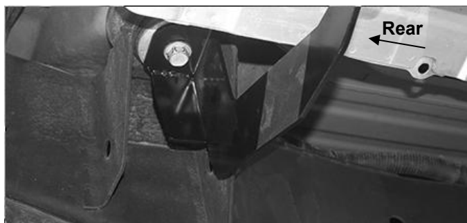
(Fig 11) Passenger side Rear Bracket Installation
