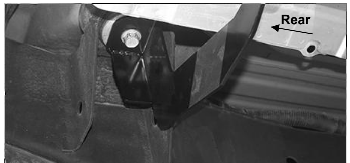
(Fig 11) Passenger side Rear Bracket Installation
