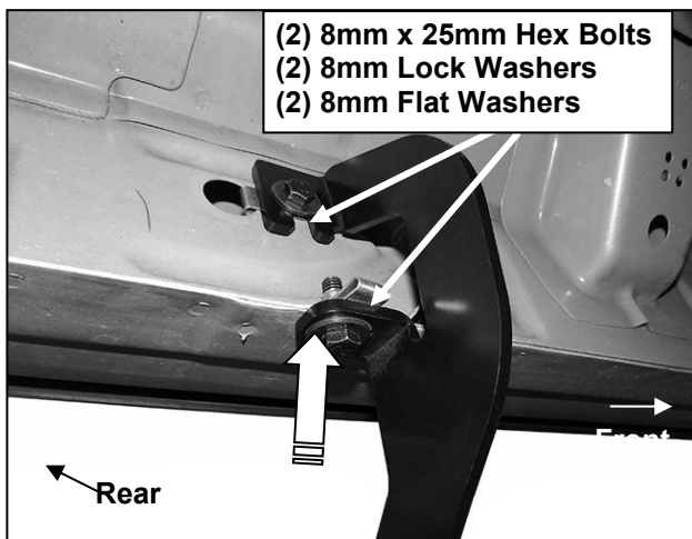
(Fig 7) Driver/left rear bracket installed
