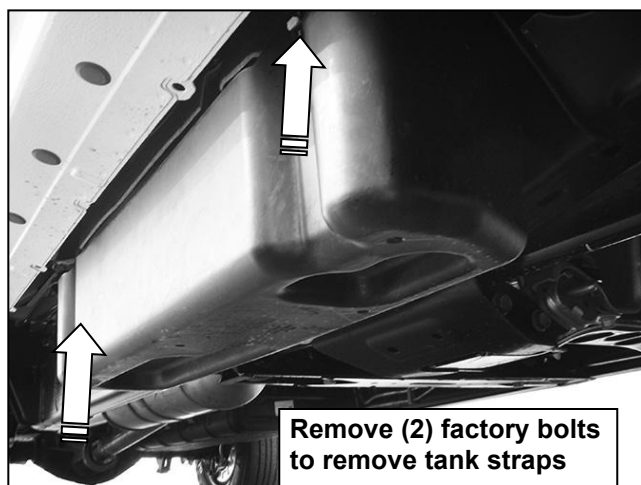
(Fig 9) Passenger side DEF tank and cover
