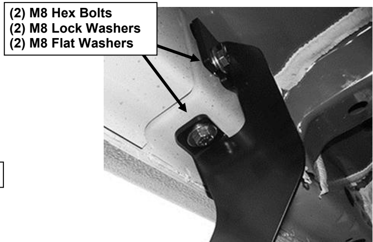
(Fig 6) Passenger side center Bracket installation
