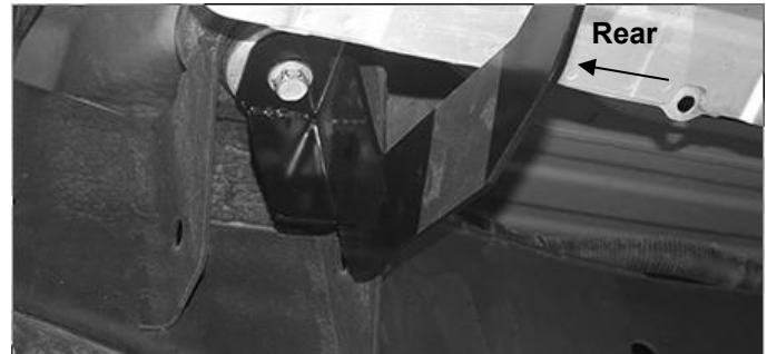
(Fig 9) Passenger side Rear Bracket Installation
