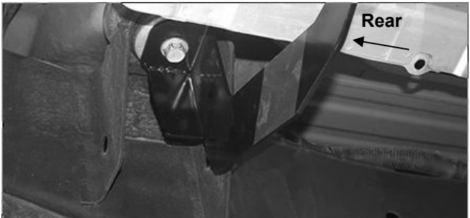
(Fig 9) Passenger side Rear Bracket Installation
